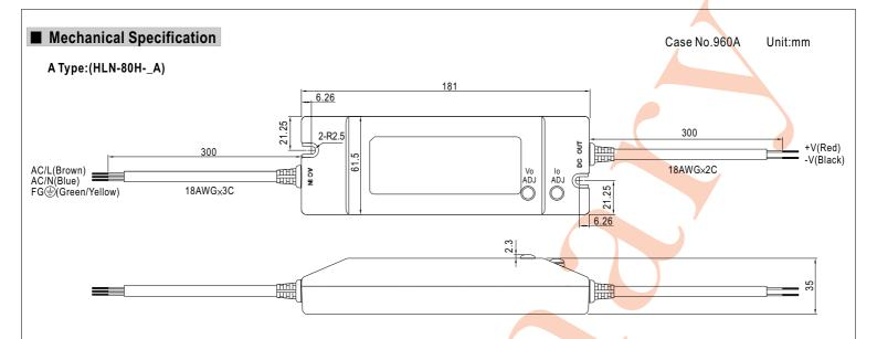
※IP64 rated. Output voltage and constant current level can be adjusted through internal potential meter. (can access by removing the rubber stopper on the case).
