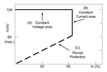
Typical LED power supply I-V curve
